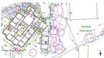
It is important to note that we have only rotate the view and NOT the model itself. If we flick back to the original view we created (which still has the Orientation parameter set to “Project North”) we see that the building is still shown orthogonally....
